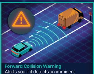
collision with a vehicle or obstacle ahead.
