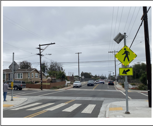
Figure 2. Example of LED-Em treatment at a pedestrian crossing. ©2022 Texas A&M Transportation Institute.
